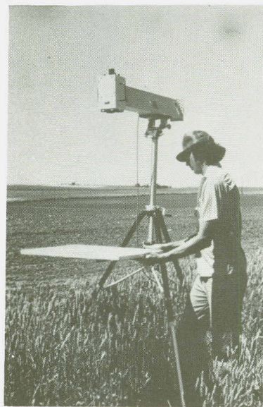
Purdue/LARS Exotech 100 tripod-mounted field system at modeling field in Williams County, North Dakota.
