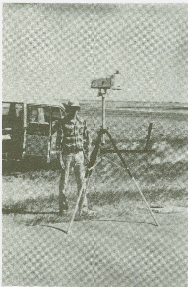
Purdue/LARS Exotech 100 tripod-mounted field system at calibration site in Williams County, North Dakota.
