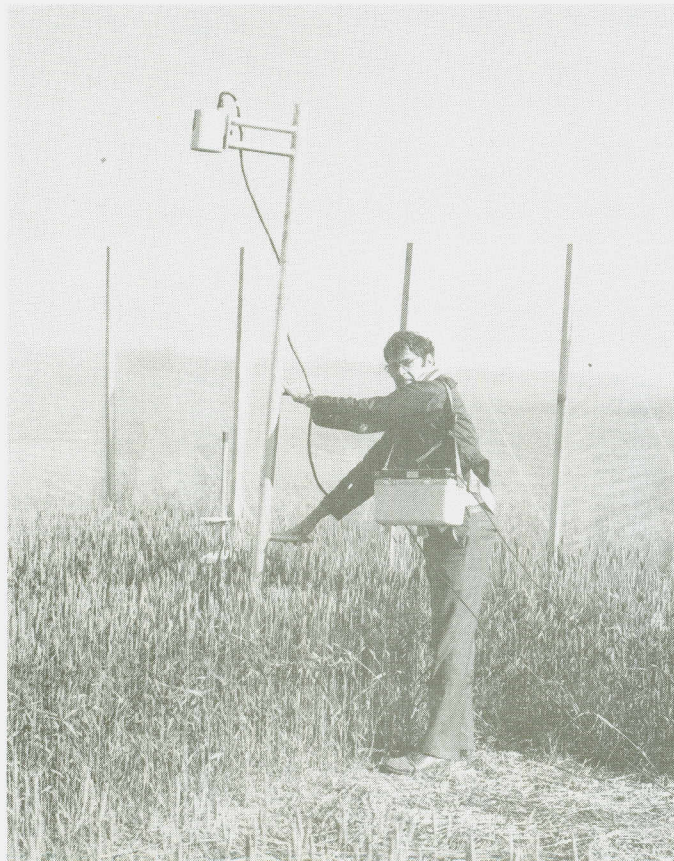
(D) Overhead Radiance Temperature measured with PRT-5 on east canopy.
